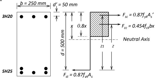
• Reinforcement used 3H20 ( $A_{s'} = 943 \text{ mm}^2$ ) and 5H25 ( $A_s = 2455 \text{ mm}^2$ ). Neutral axis depth,
