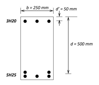
Chac. strength of concrete  $f_{ck} = 30 \text{ N/mm}^2$
